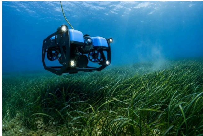
Fig. 6.1.4 Monitoring of the upper and lower limits of Posidonia oceanica meadows using a remotely operated vehicle (ROV).
